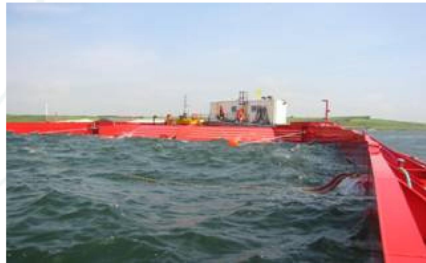
Wave energy converter, 20 kW prototype WAVE DRAGON project
